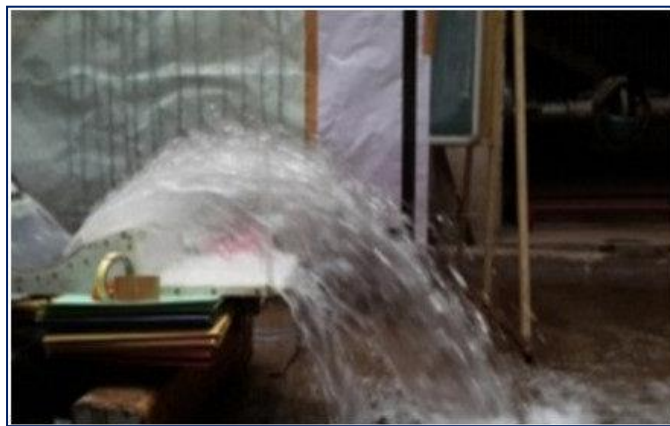
Glimpses of model of roller bucket energy dissipater in fluid mechanics lab
